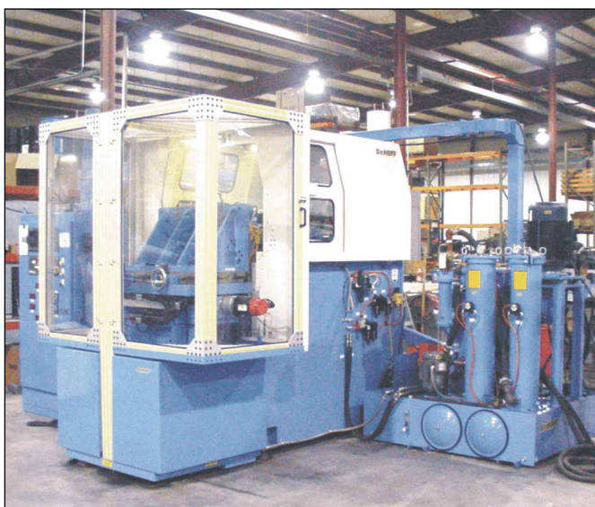
Twin spindle CNC Knee Gundrill Center .005mm positioning accuracy, 24,000 RPM spindles
